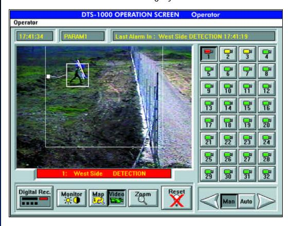
DTS-1000 provides advanced digital video intrusion detection and tracking on a Personal Computer platform. The system operates with an array of commercially available CCTV cameras which are strategically placed to provide overlapping visual coverage of the protected site.
